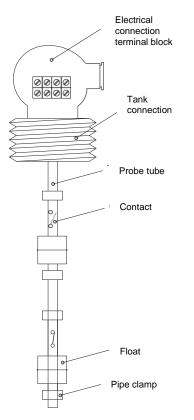
These probes are designed to be mounted from the top of the reservoir.
