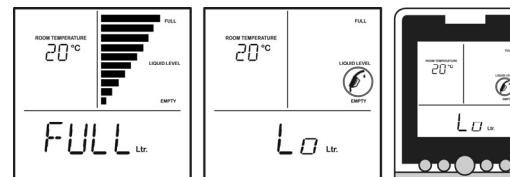
When the tank level is such that there is below 10% of the usable volume of oil left in the tank, the CURRENT information screen alternates between showing the 'Ltr.' (or % or DTE) and 'Lo'. If the level then drops such that there is below 5% of usable oil left:
