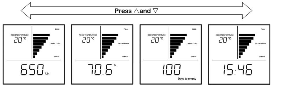
For approximately 1 week after the Tankalert Eco Oil is installed, it collects data so that the 'Average per day' value may be calculated. During this period the screen will flash '—' when showing 'Days to empty'. (In the picture 'flashing' is indicated by the red circle).
