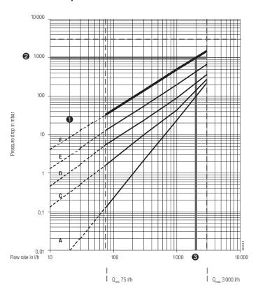
Mineral oil, viscosity 450 mPa.s VZO 25 mounted on pressure side of pumps
